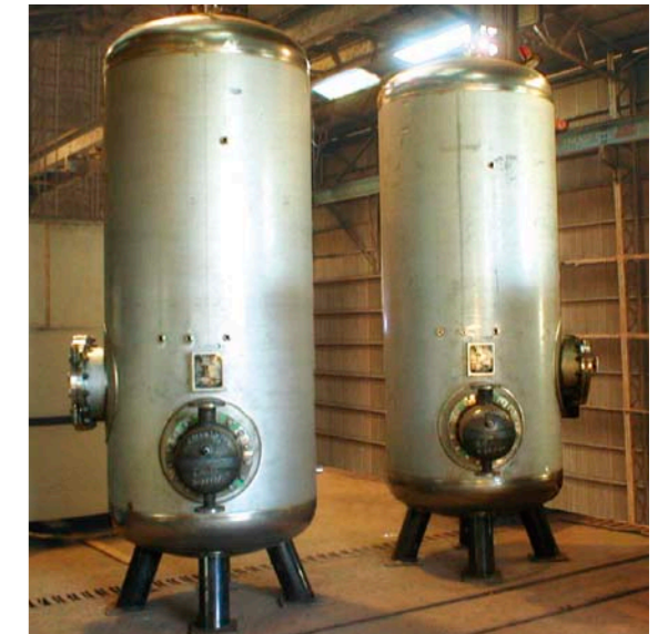
Hot water tanks (SUS444, NSSC190L)
